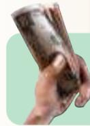
A liner made from HDPE would have to be 60 mils thick, which equals a stack of 60 garbage bags. The construction cost can be as high as \$750,000 per acre.
