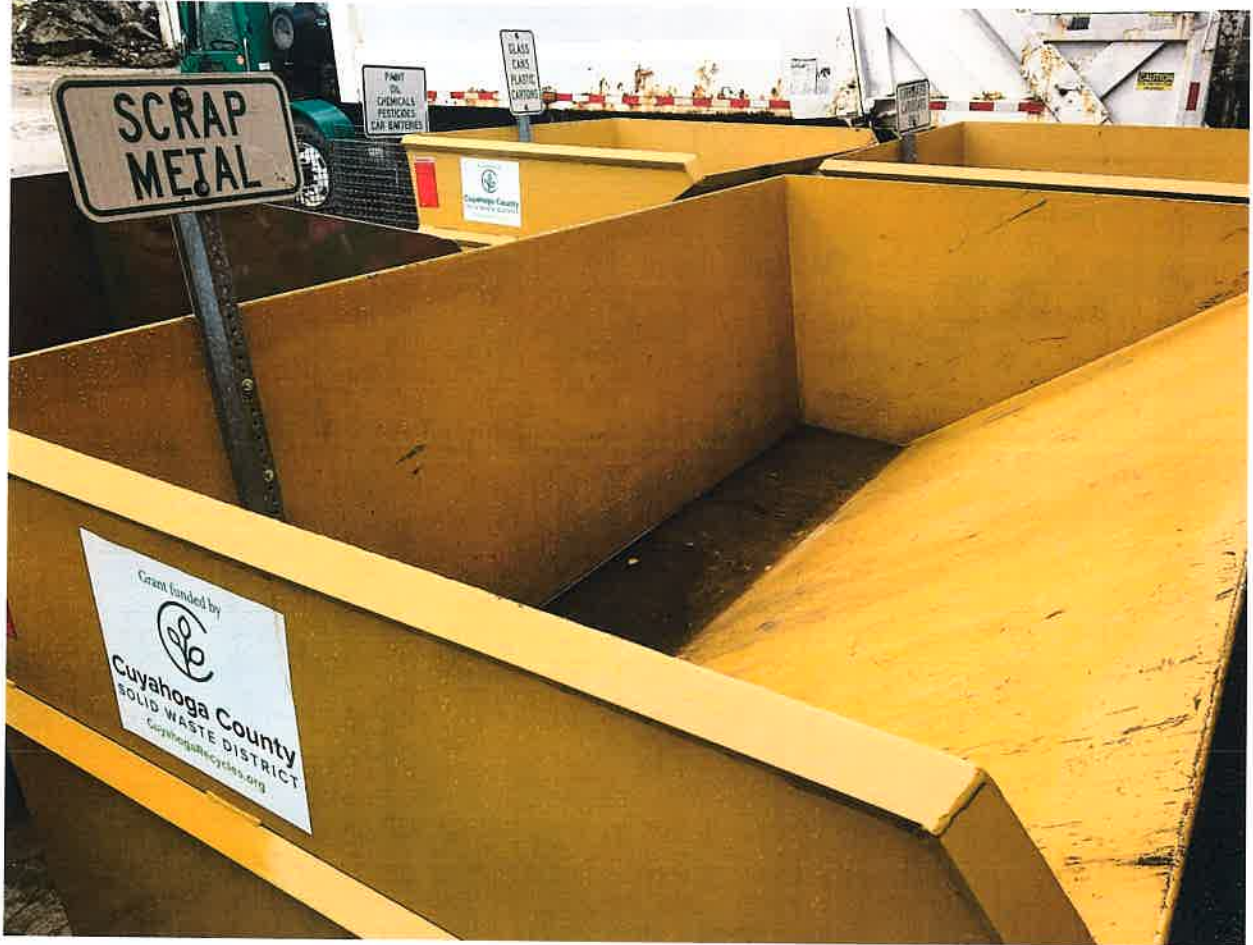
The new 5 Cubic Yard Lift Truck Hopper is used for the collection of Scrap Metal at the Brecksville Recycle Center.
